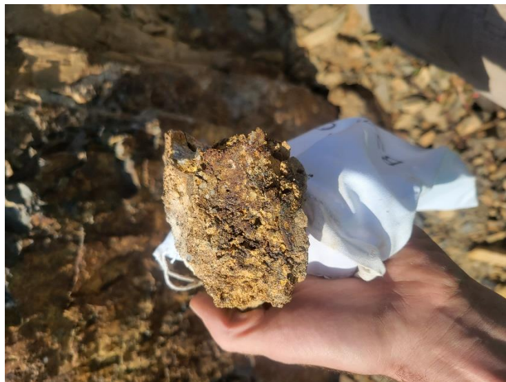
Figure 7: Surface Geology Mapping: Crusher Zone South – Strong FeOx alteration with jarosite and silicification developed along fault
