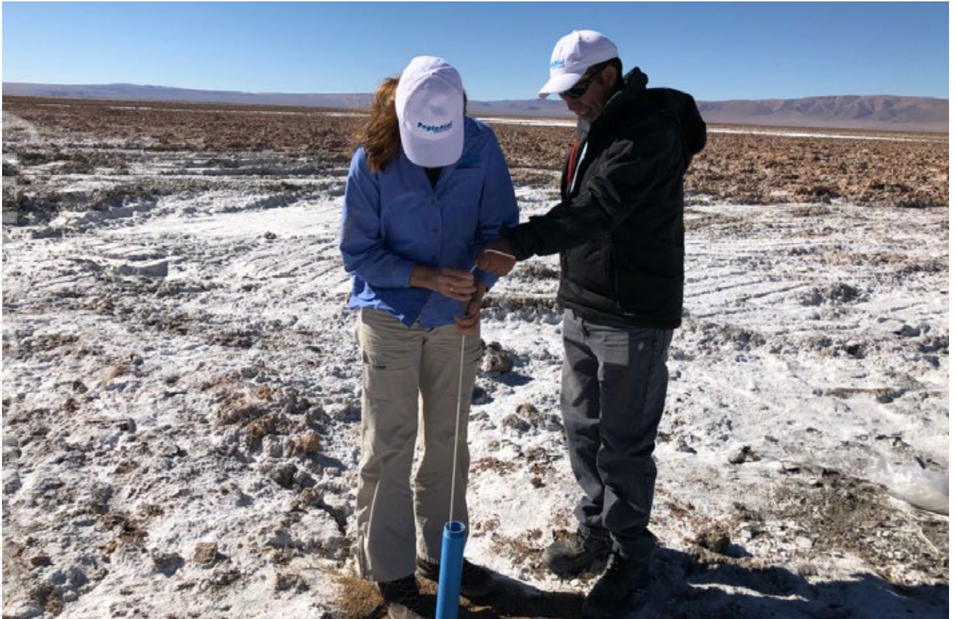
Photo 2 – Salar de Rincon - Brine was pumped from monitoring wells converted from resource drilling program Dec 2017
