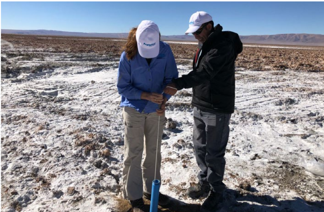
Photo 2 – Salar de Rincon - Brine was pumped from monitoring wells converted from resource drilling program Dec 2017
