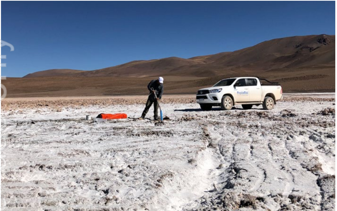
Photo 11 – Monitoring Brine Level - Salar del Rincon
