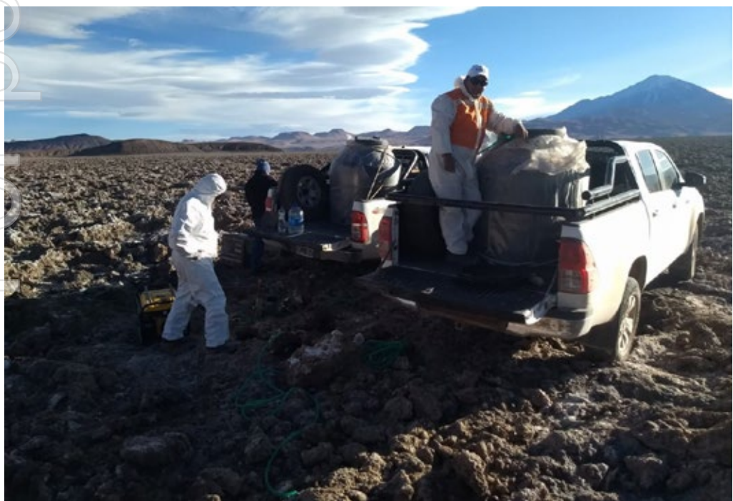
Photo 1 – Salar de Incahuasi - Brine Collection by pumping from trenches created Aug-Sep 2019
