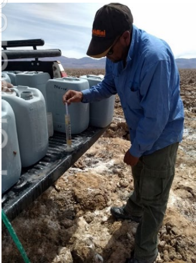
Photos 3 and 4 – Relative density of brine measured before and labelled plastic brine containers were sealed for transport
