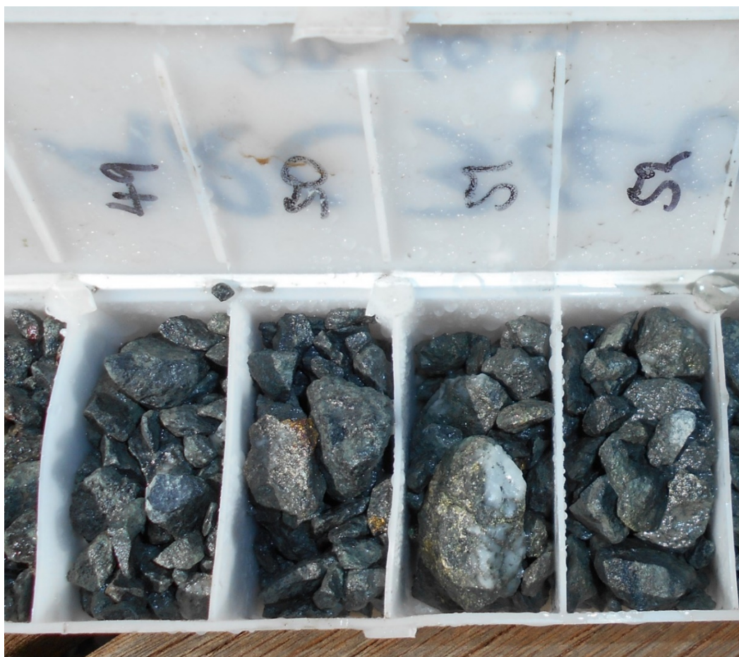
Figure 3: Hole ARC340 (49-51m) 5% sulphides comprising pyrite and chalcopyrite with quartz carbonate veins, located in the Crosscut Zone.
