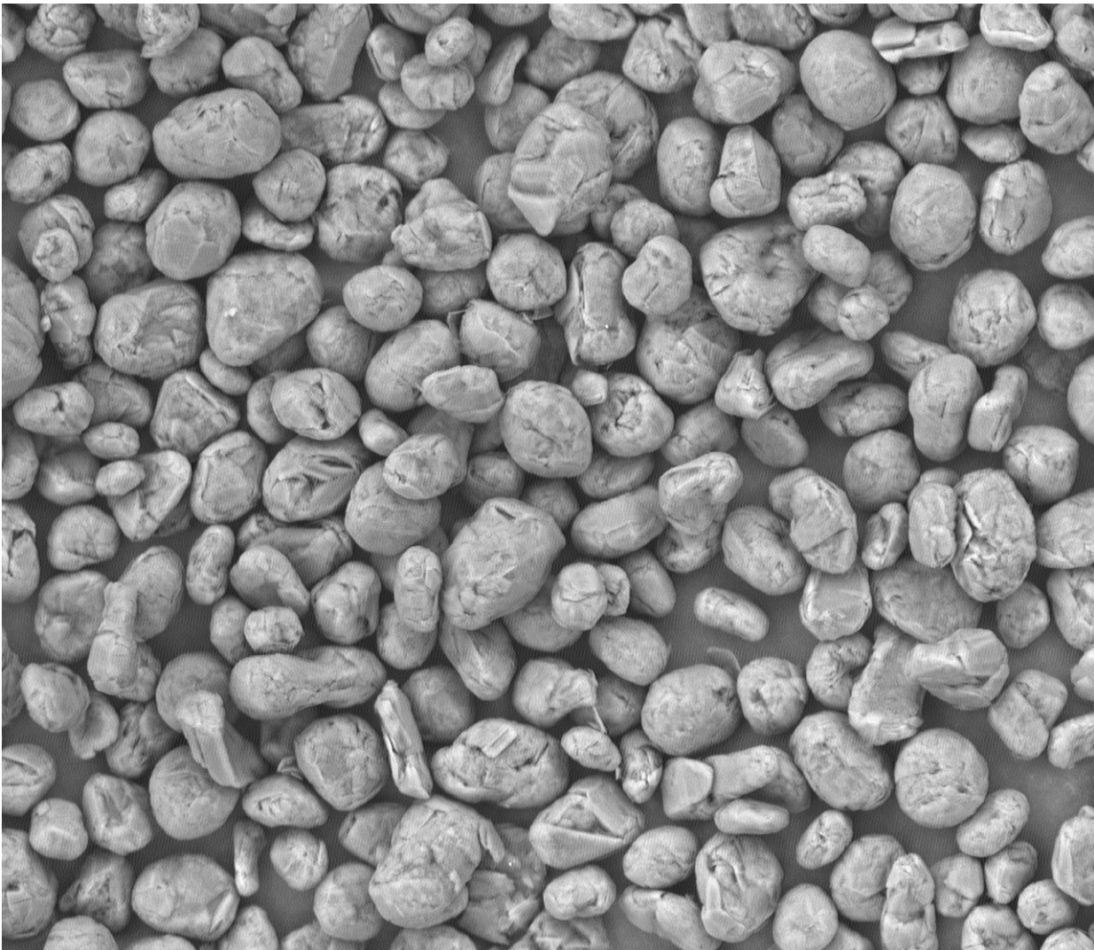
Picture 1: SEM image of 20 micron spherical graphite
