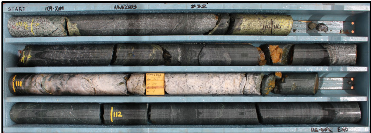
Image 7 | NWD2003: 109.2m to 110.05m; 0.7m @ 6.58% Cu, 2.83 Au g/t and 16.5 g/t Ag.
