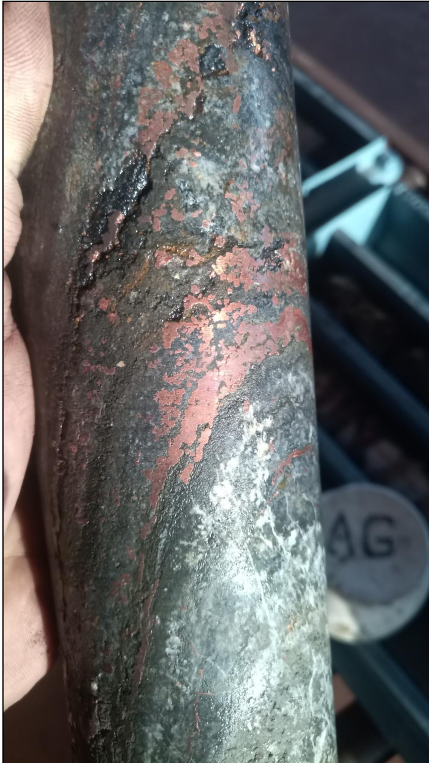
Image 3 | Hole 21NDMT001: 150.3m to 150.5m showing native copper, covellite, chalcopyrite and chalcocite
