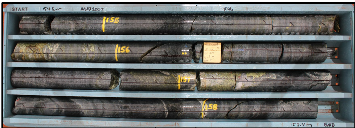
Image 8 | NWD2003: 155.0m to 156.0m; 1.0m @ 5.11% Cu, 0.40 Au g/t and 8.50 g/t Ag, 156.7m to 157.4m; 1.0m @ 11.0% Cu, 0.82 Au g/t and 18.5 g/t Ag.
