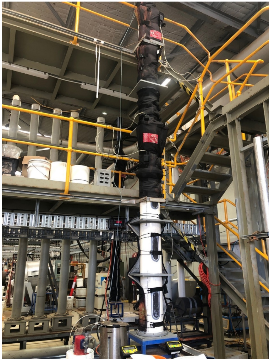
Image 4 | Nifty 6m high metallurgical testwork column
