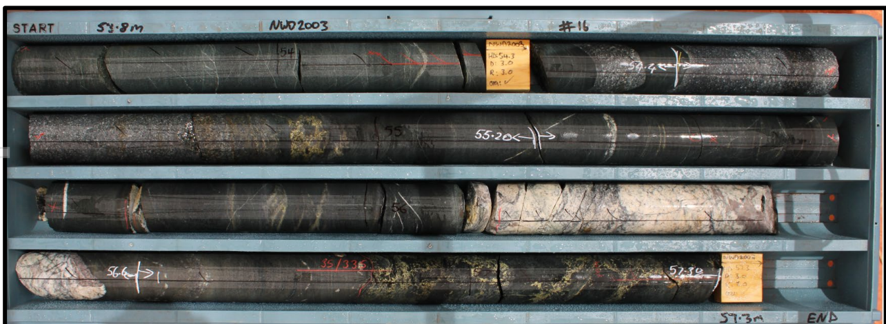
Image 6 | NWD2003: 56.6m to 57.3m; 0.7m @ 3.12% Cu, 0.33 Au g/t and 6.00 g/t Ag.
