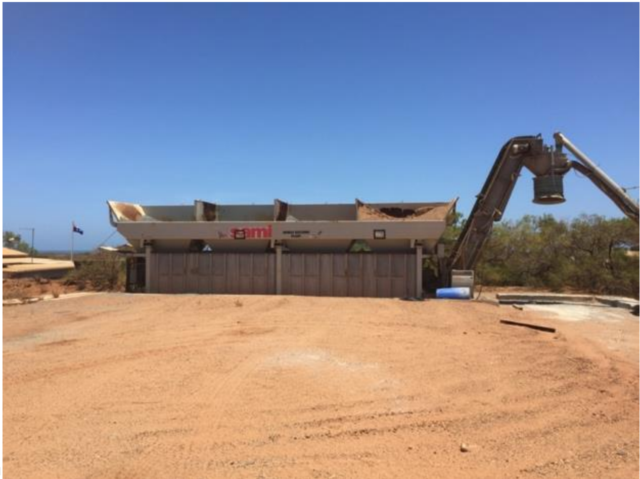
Figure 6: T4 Sami Mobile Concrete Batching Plant, Lot 697 Cornish Way, Onslow
