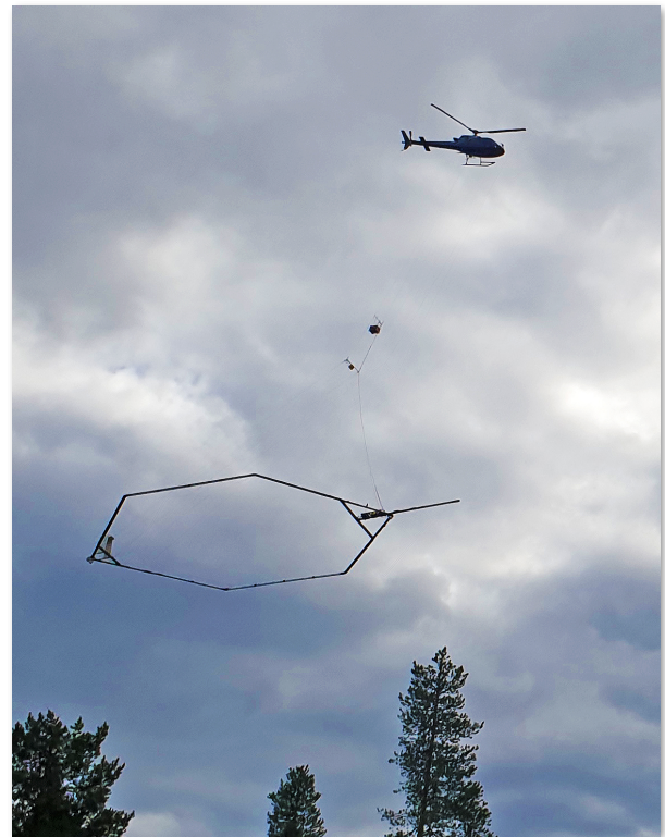
Figure 1 SkyTEM system airborne on Talga project.
