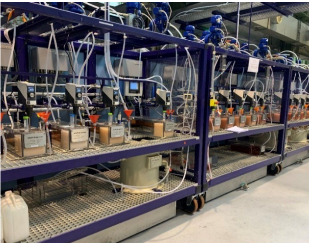
Figure 2 – Refining circuit – nickel extraction
