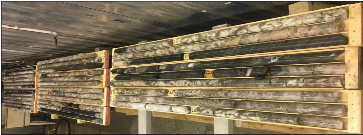
Figure 8: Drill hole MF18-53 including internal waste returning 55.25m at 1.04% Li 2 O from 82.75m
