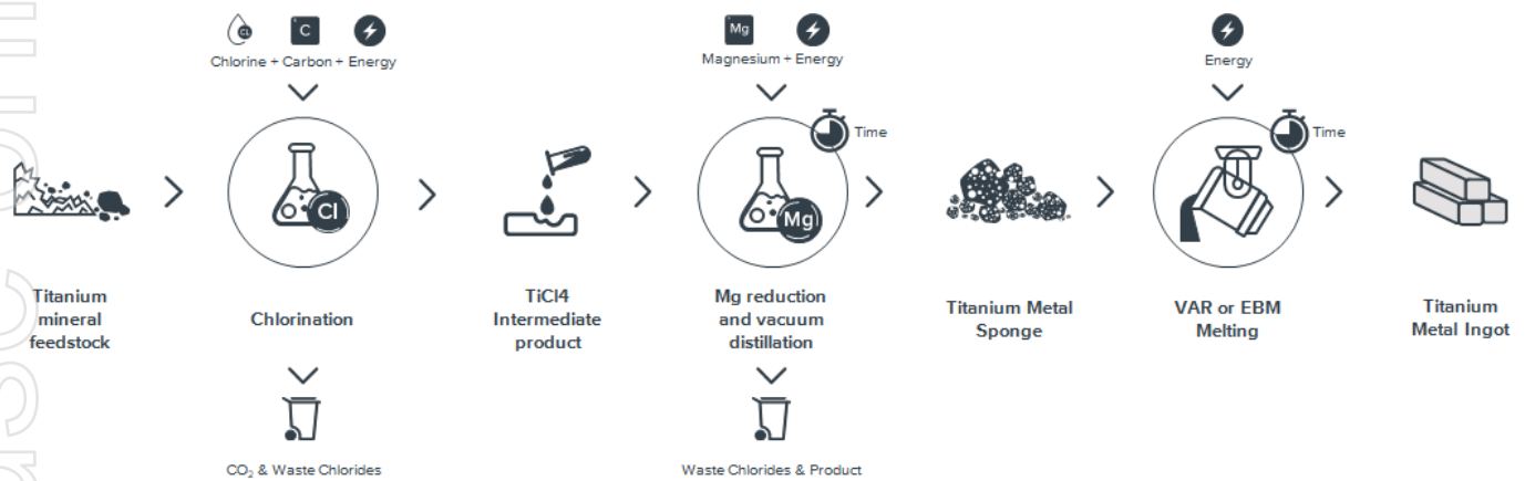
Figure 1: Current titanium metal manufacturing process diagram.
