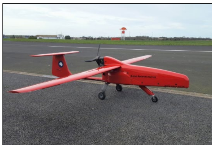
Figure 3: The Prion Mk3 drone used for the magnetic survey
