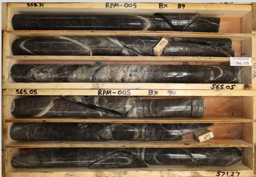
Figure 3c. RPM-005 drill core interval 170-174 meters (558.31-571.27 feet) depth returning 97.8 g/t Au . Typical mineralized structure and veining within intercalated hornfels (dark) and qtz-feldspar intrusive dyke (light) host rocks.
