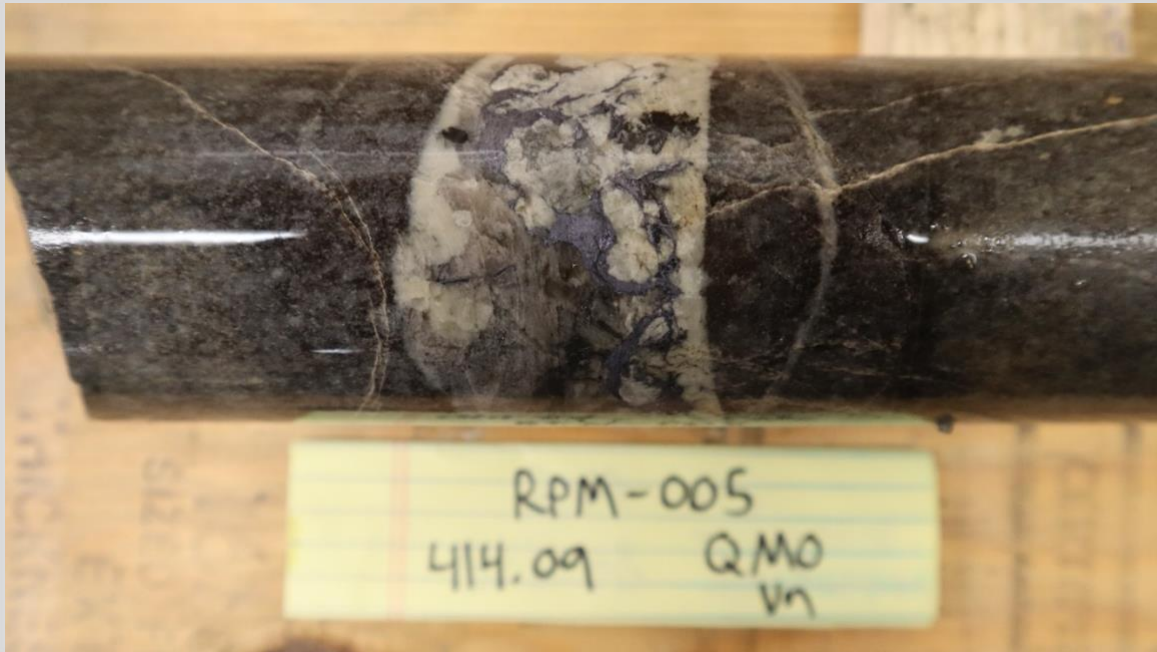
Figure 4a. RPM-005 selected core showing Au bearing qtz-moly veining at 126.2 meters (414.09 feet) depth from sample interval returning 41.8 g/t Au .
