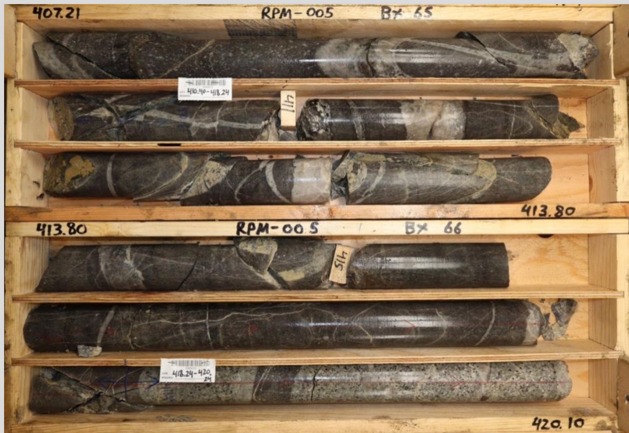
Figure 3a. RPM-005 drill core interval at 124-128 meters (407.21-420.10 feet) depth returning 41.8 g/t Au.
