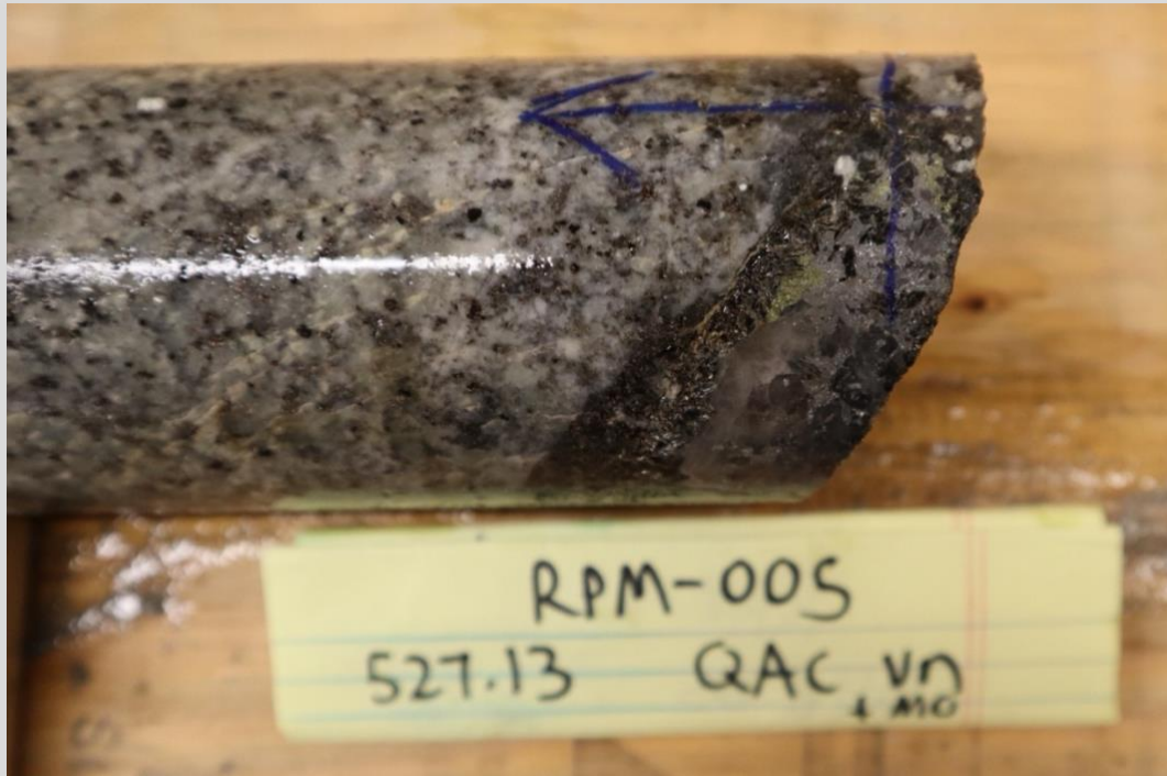
Figure 4c. RPM-005 selected core showing qtz-arsenopyrite-chalcopyrite vein hosted in qtz-felspar intrusive at 160.7 meters (527.13 feet) depth within sample interval returning 50.3 g/t Au.
