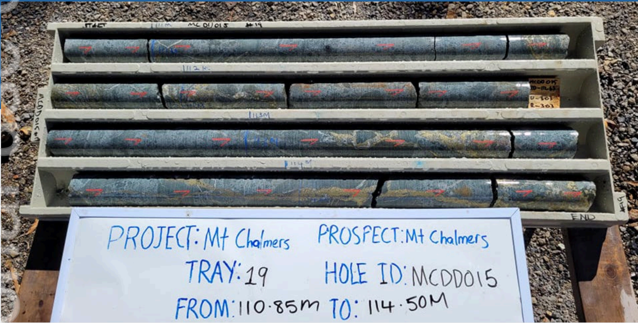
Figure 9: MCDD015 Tray 19 (110.85m to 114.50m) showing mineralised stringer zone chalcopyrite veining in felsic pyroclastic footwall breccia.
