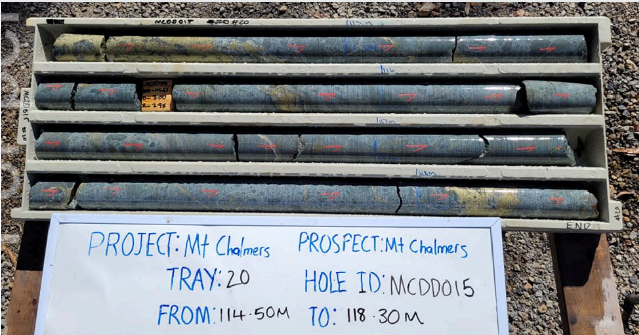
Figure 10: MCDD015 Tray 20 (114.50m to 118.30m) showing mineralised stringer zone chalcopyrite veining in felsic pyroclastic footwall breccia.
