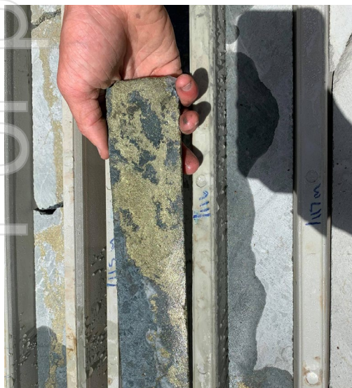
Figure 1: Drill Hole MCDD015 Showing Chalcopyrite Stringer Veins.
