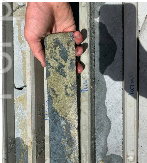
Figure 1: Drill Hole MCDD015 Showing Chalcopyrite Stringer Veins.
