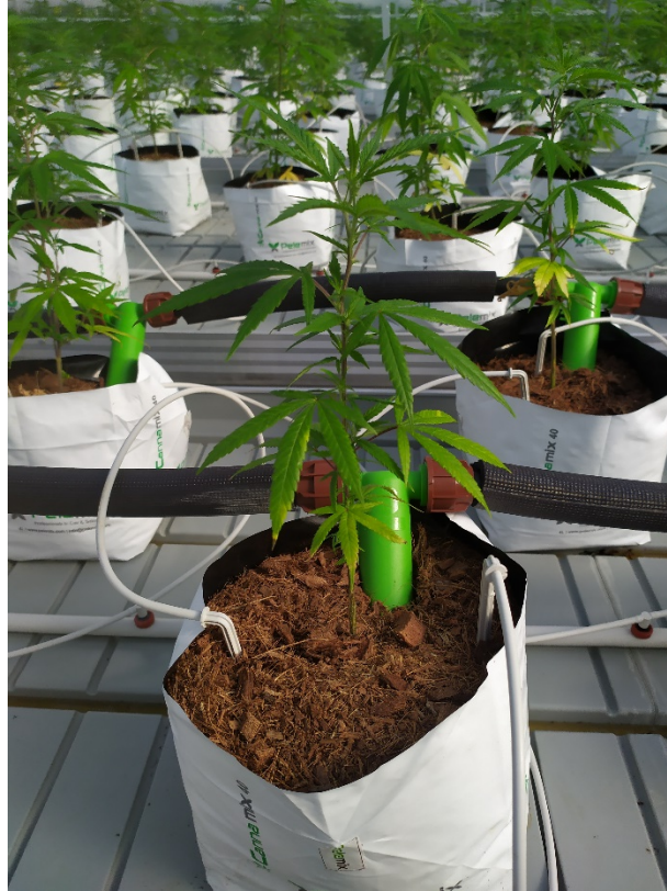
Image: Roots' Heat Exchange Probe deployed into grow bags
