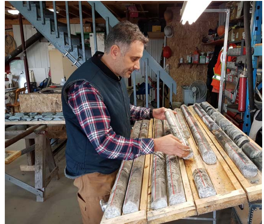
Drill core from drilling at the Tansim project
