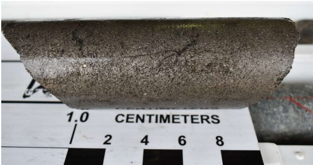
Figure 4: Massive sulphides 21WDD0004 130.5m downhole, pyrrhotite with smaller "shinier" pyrite and chalcopyrite (greenish)
