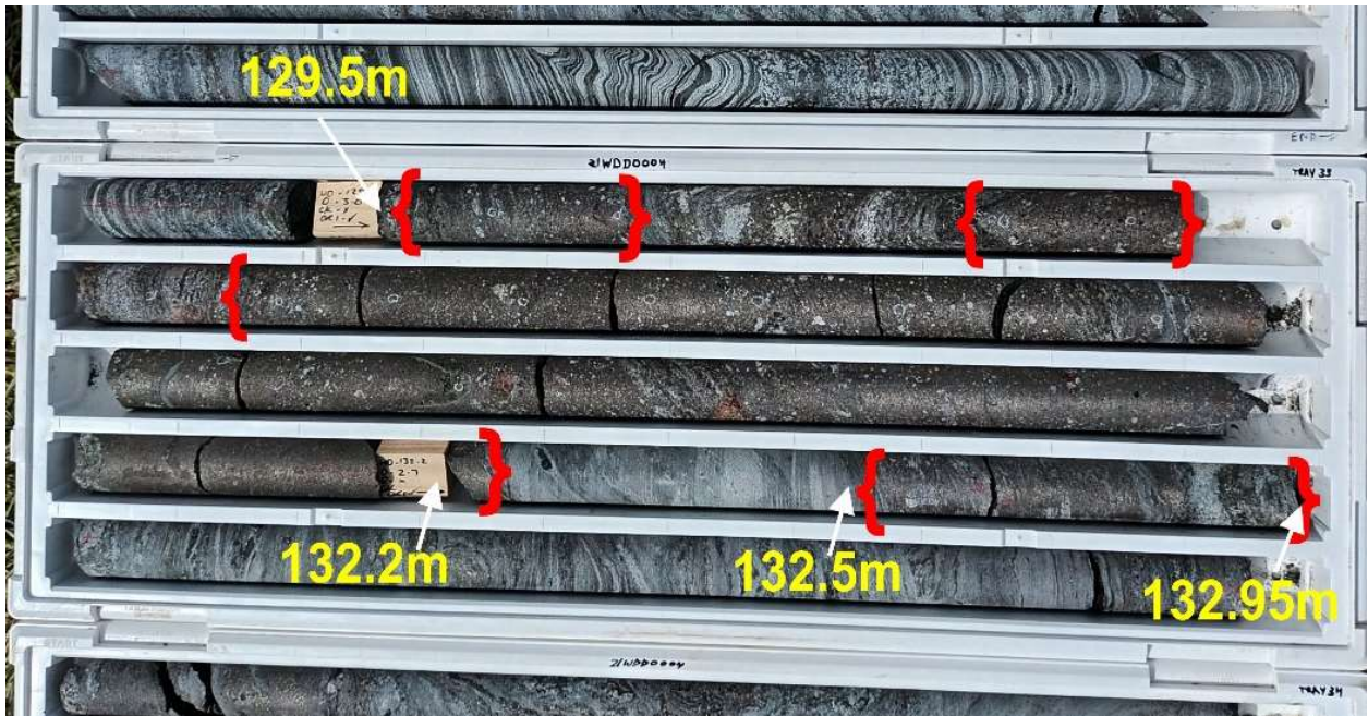
Figure 1: Drill Core from 21WDD0004 showing massive sulphide bands (red brackets)
