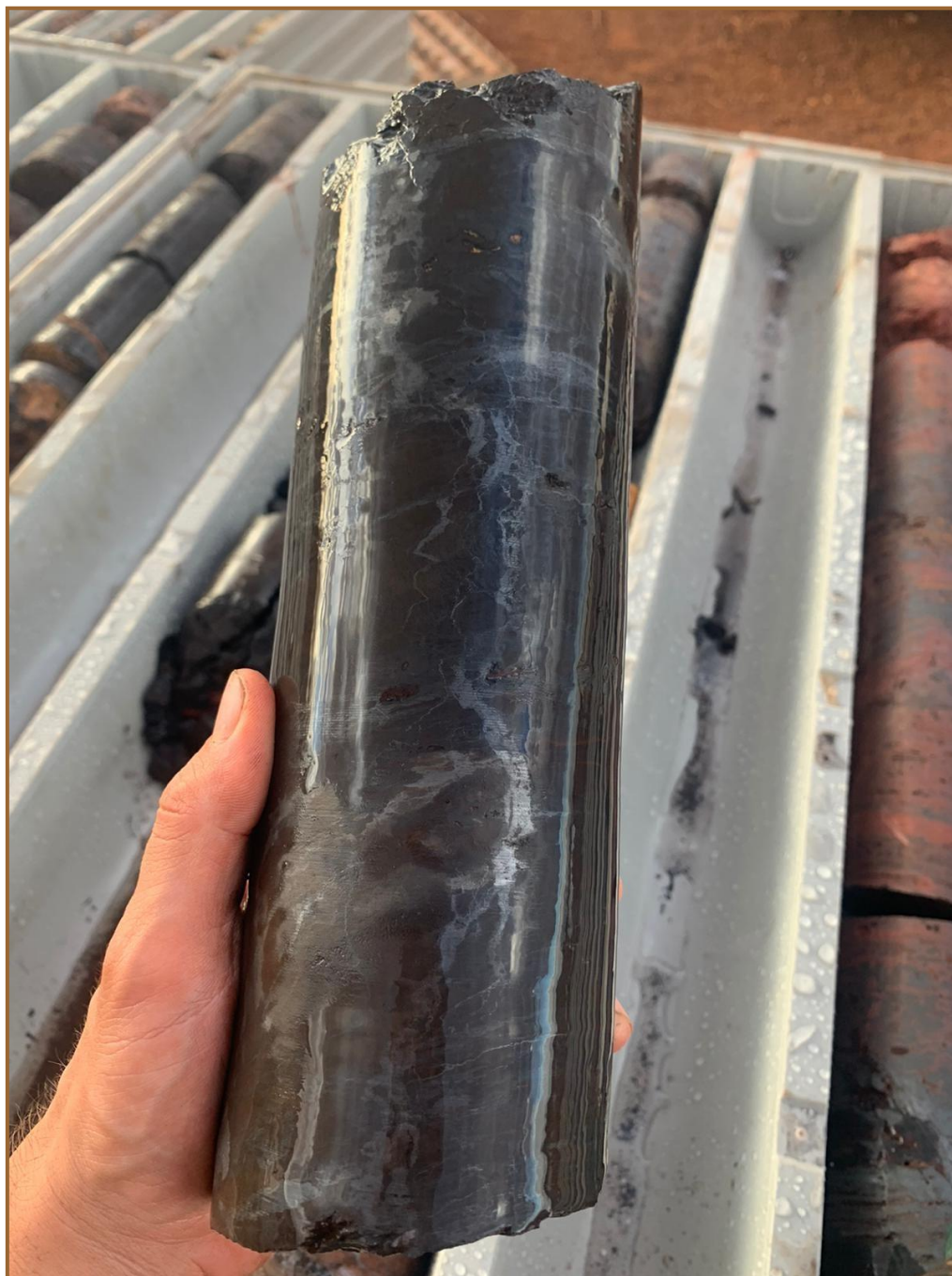
Plate 1 – ~40% Manganese core from BRDD005 (10.2m – 10.4m)
