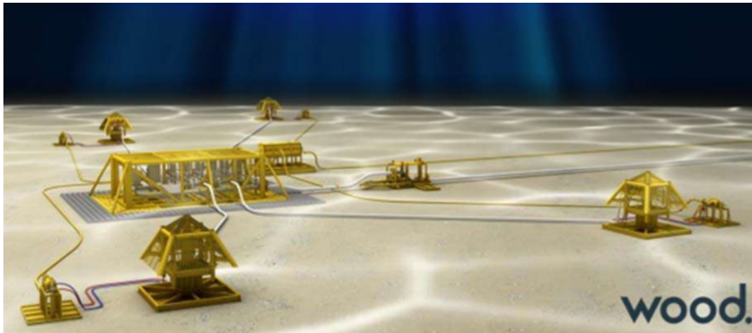
Figure 7: Indicative Image of 4 x Well Subsea Completion Facilities (Image provided courtesy of APA)
