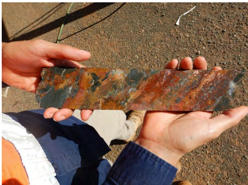
Figure 9: Hole 21CCDD003 122.36 - 122.66m chloritic altered brecciated basalt host with ~5% native copper with moderate to strongly oxidised limonite-goethite
