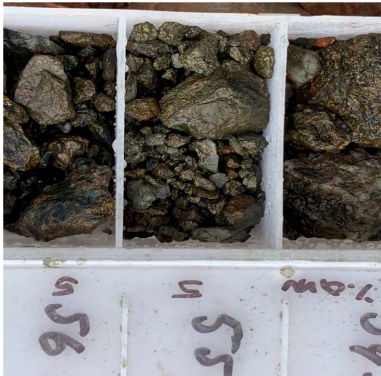
Figure 8: Chalcopyrite/pyrite in silicified and sericite altered basalt host. Grade for this interval returned 6m @ 14.97g/t Au, 7.09% Cu and 0.06% Co, from 53 metres in Hole ARC310.
