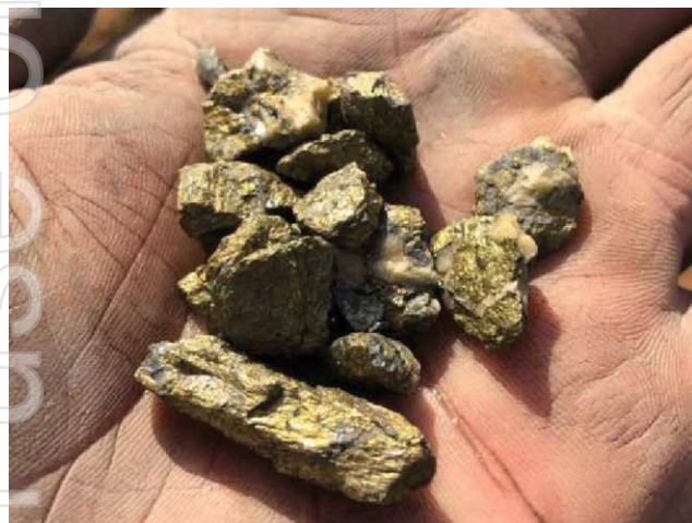
Figure 4a (left). Rich Chalcopyrite Mineralisation (88-89m, 5.8% Cu – WCRC021); and Figure 4b (right). Rich Chalcocite Mineralisation WCRC006 (18-19m) at Powder Hill, Grading 9.5% Cu .
