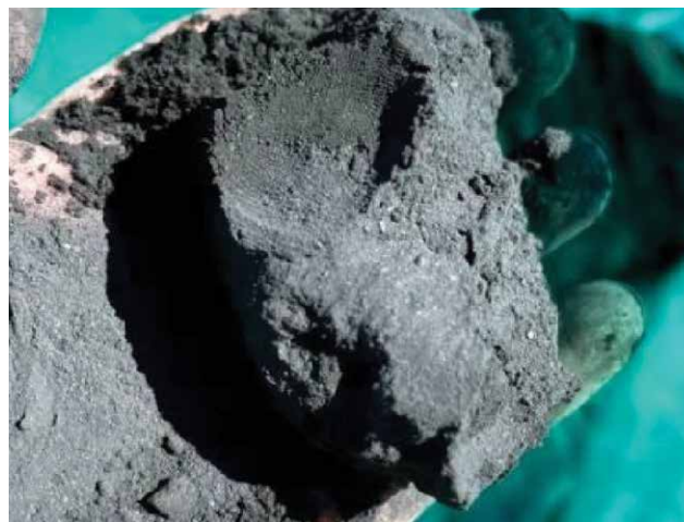
Figure 4a (left). Rich Chalcopyrite Mineralisation (88-89m, 5.8% Cu – WCRC021); and Figure 4b (right). Rich Chalcocite Mineralisation WCRC006 (18-19m) at Powder Hill, Grading 9.5% Cu .
