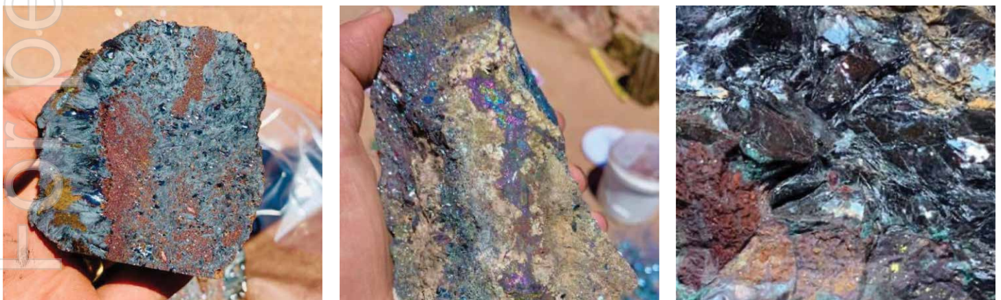
Figure 14. IOCG mineralisation in hematite-breccias, outcropping at the Flinders Project.
