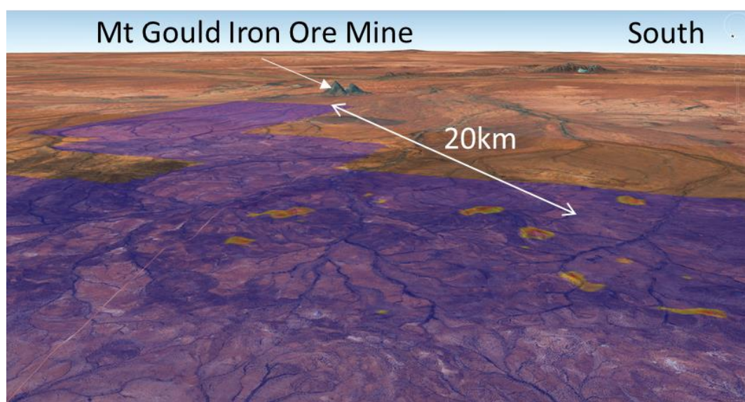
Figure 7 Dingo Pass Airborne EM anomalies. Modelling of Ground EM traverses has produced causative plates of very high conductance.
