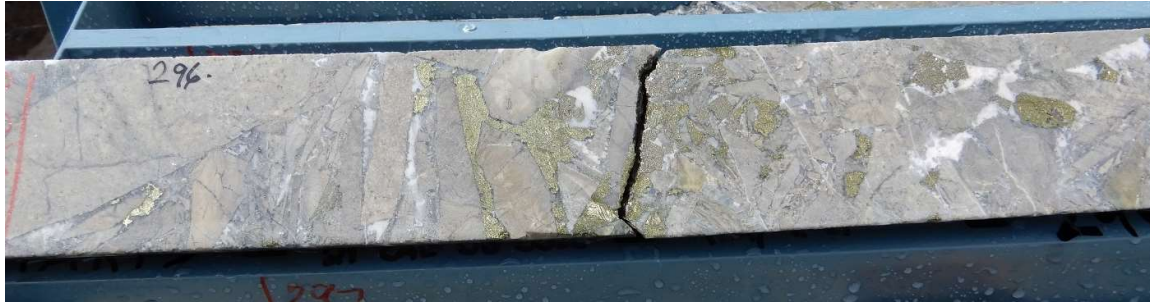
Fig 16. Primary copper mineralisation Hole 21CAEDD002 , 296m , -8% visual estimate of chalcopyrite in the interval 296m-297m,, Assay results awaited.
