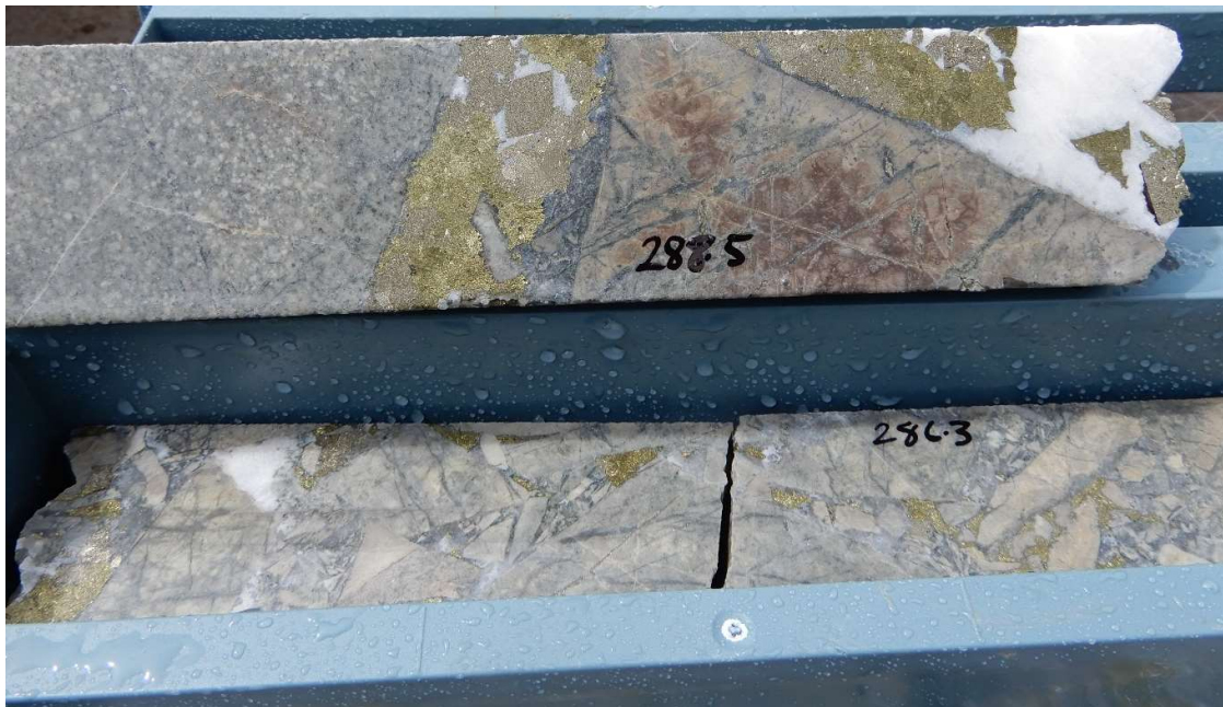
Fig 14. Primary copper mineralisation Hole 21CAEDD002, 288.5m , -5% visual estimate of chalcopyrite in the interval 288m-289m, Assay results awaited.
