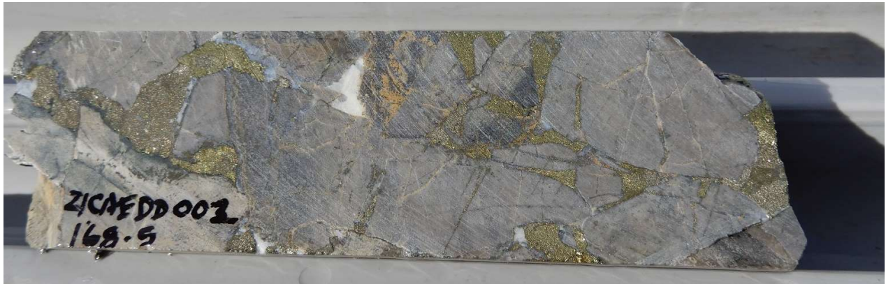
Fig 11. Primary copper mineralisation Hole 21CAEDD002 ,168.5m , 4% visual estimate of chalcopyrite in the interval 168m-169m. Assay results awaited.
