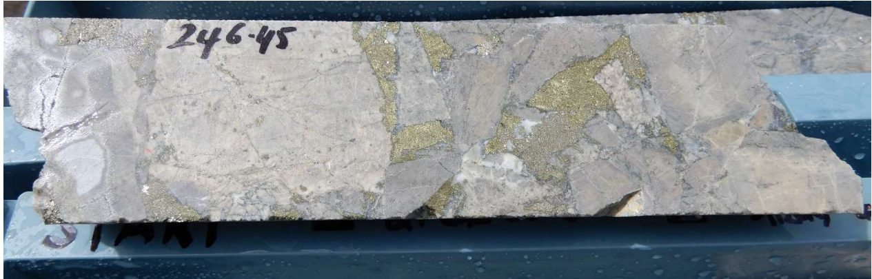
Fig 13. Primary copper mineralisation Hole 21CAEDD002 , 246.45m , -3% visual estimate of chalcopyrite in the interval 246m-247m, Assay results awaited.
