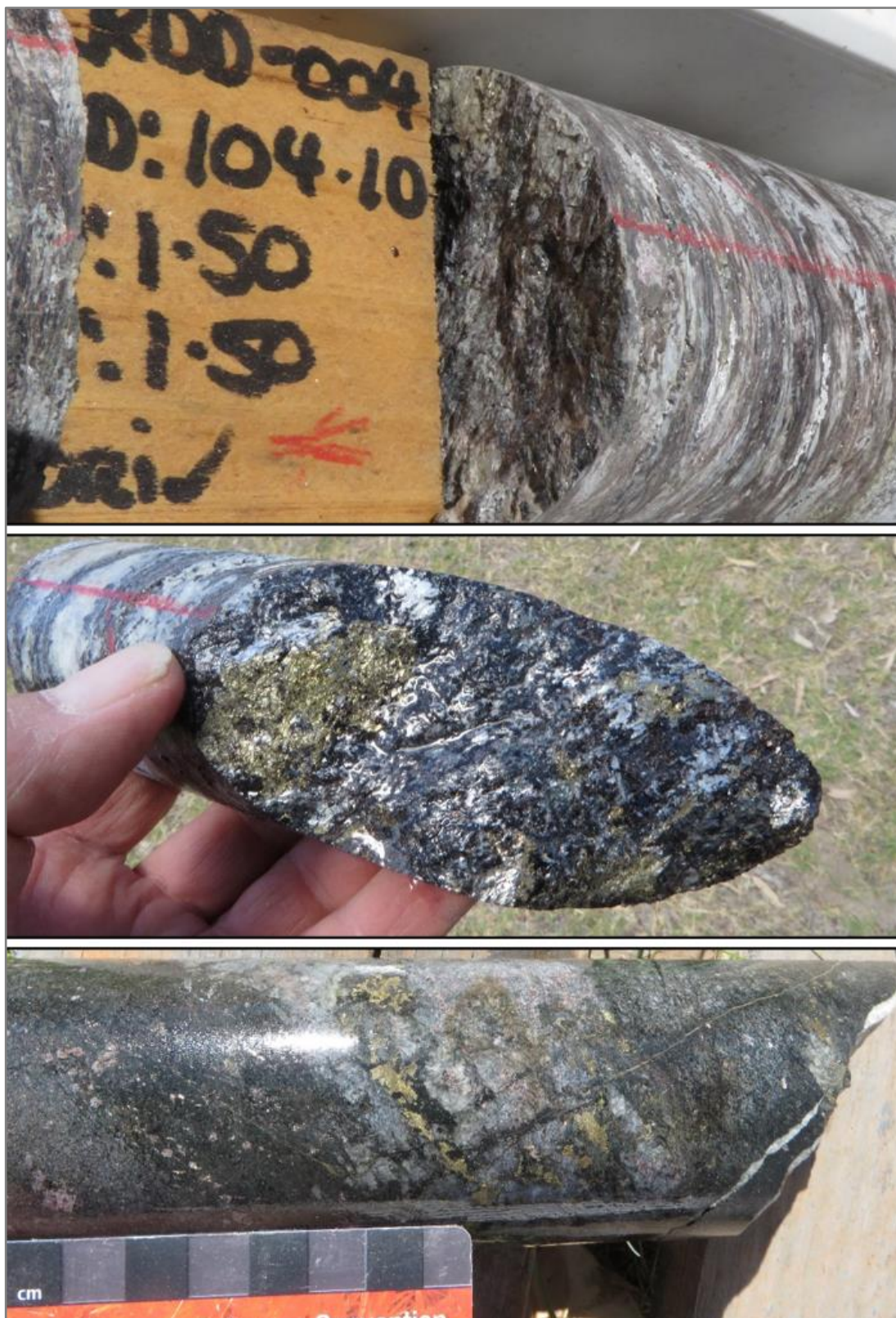
Source: Dalaroo, July 2021. Examples of muscovite-chlorite-pyrite alteration. Top – Pale-silvery-white muscovite defining cleavage seams, LRDD004 104 m depth. Middle – Film-like aggregates of fine pyrite intergrown with muscovite on a cleavage seam, LRDD004 120 m depth. Bottom – Fine quartz veinlets cutting biotite schist and a K-feldspar replacement vein, with feldspar replaced by chlorite in a narrow selvage and coarse euhedral pyrite intergrown with chlorite along the replacement vein.
