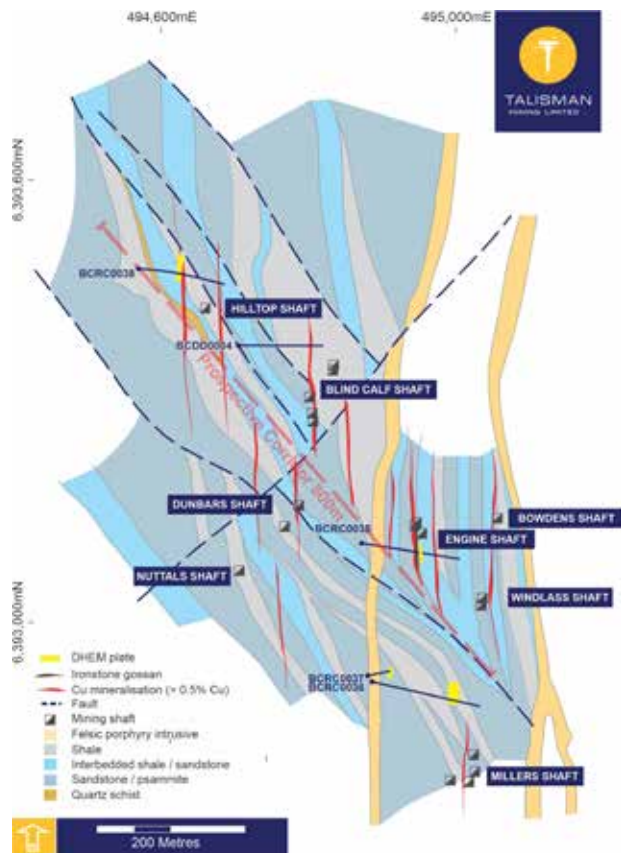
Figure 7: Blind Calf Prospect geological interpretation showing recent drilling, tested down-hole EM (DHEM) conductors and drill holes 10 proposed for DHEM surveys.
