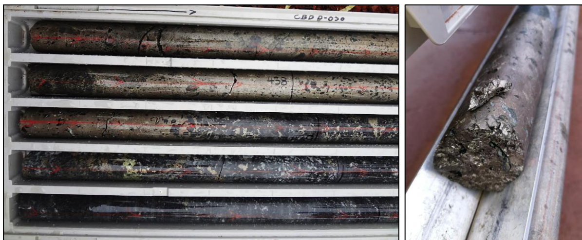
Figure 3: Ni-Cu bearing massive sulphide zone in diamond drill hole CBDD030 drilled 300m south of the T5 Ni-Cu discovery zone.
