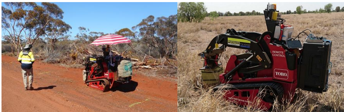
Figure 5: R&D Seismic Survey conducted by Ultramag enabled very low environmental impact seismic surveying at Carr Boyd, allowing the company to image the prospective basal contact at depth ahead of drill planning.
