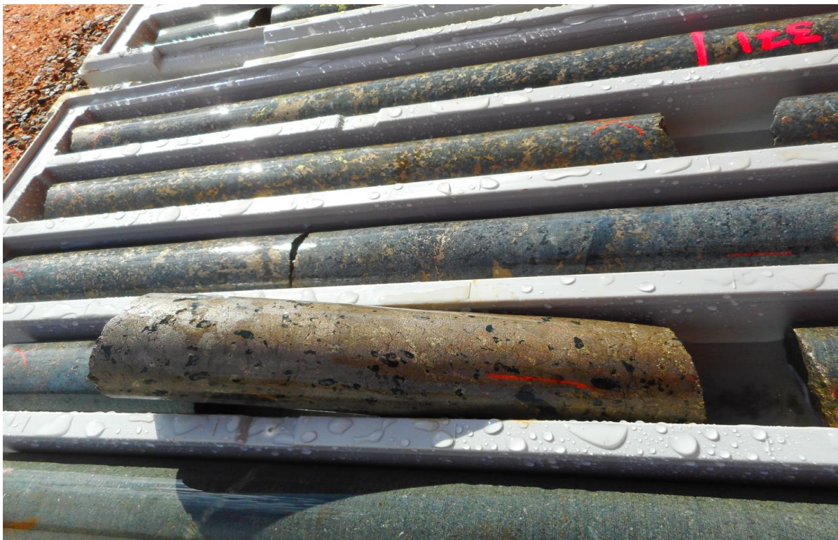
Figure 9: Massive and globular nickel sulphides from CBDD054B. The globular sulphides sit atop the massive and represent active erosion of the massive sulphides by the crystallising melt.
