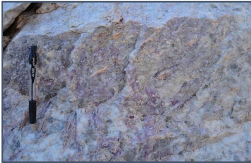
Figure 4: An example of mineralised D0 pegmatite clearly showing spodumene crystals 4
