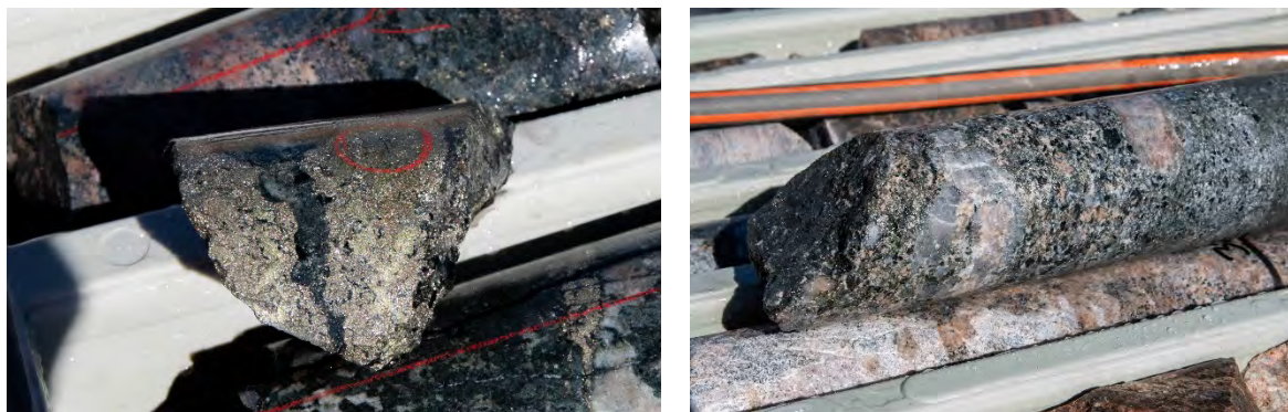
Mineralised zone in EHRCD003 (329.6 m -329.8 m) – Pyrite dominant with lesser chalcopyrite
