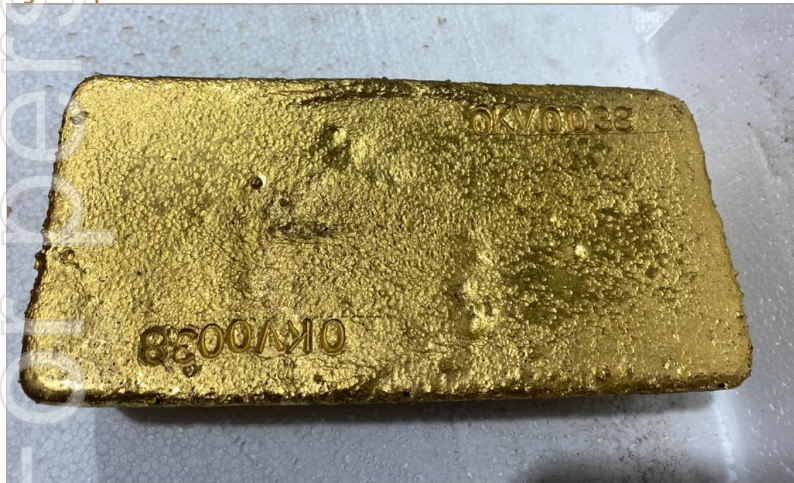
Figure 3 | Gold Doré Bar No OKV0038 of 634oz Poured at the Okvau Gold Mine
