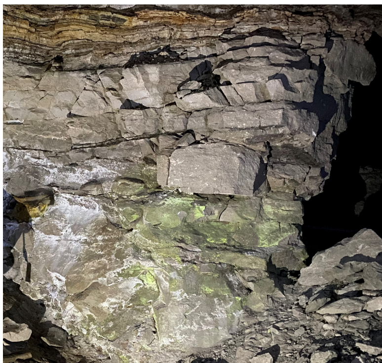
Figure 2: Photo of visible uranium and vanadium mineralisation associated with high-carbon stratification and localised remobilisation within historical underground workings of the Yellow Cat project.
