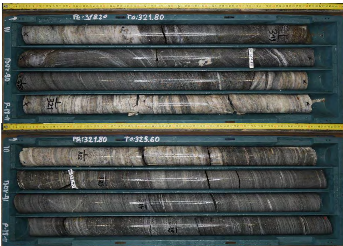
Picture 5: Pegmatite intersection of drill hole P18-11 @ 322m with a true thickness of 1,60 m
