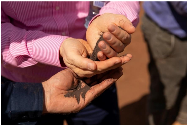
Left: Examining proppant used for fracture stimulation at the Carpentaria-1 well site
