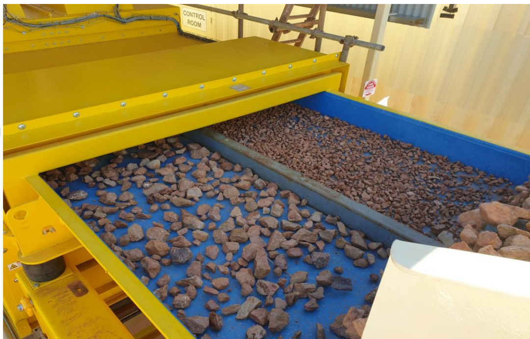
Figure 2: Feeder with simultaneous feed of two size fractions of ore to the ore sorter machine
