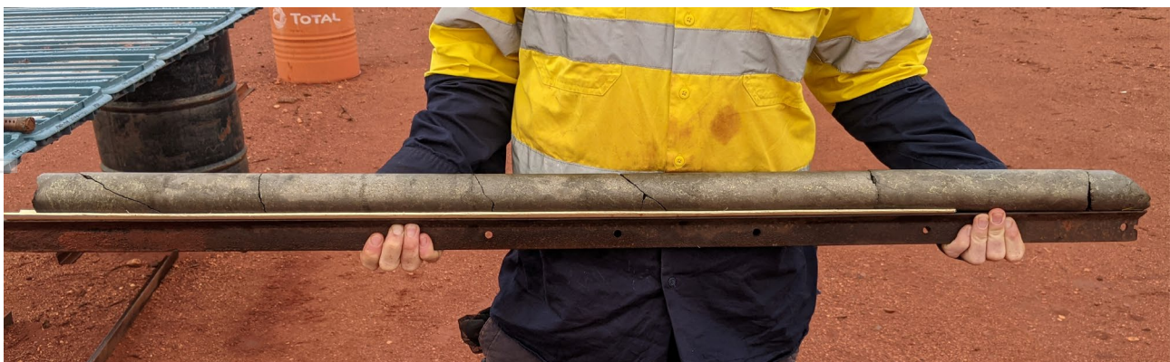
Figure 4 – f resh drill core from the massive sulphide interval of MAD199 between 342.12m to 343.4m.
