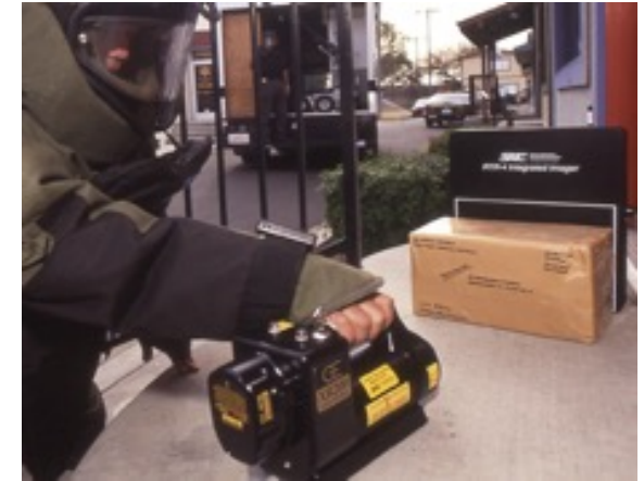
Traditional x-ray of IEDs requires manual placement of separate detector
