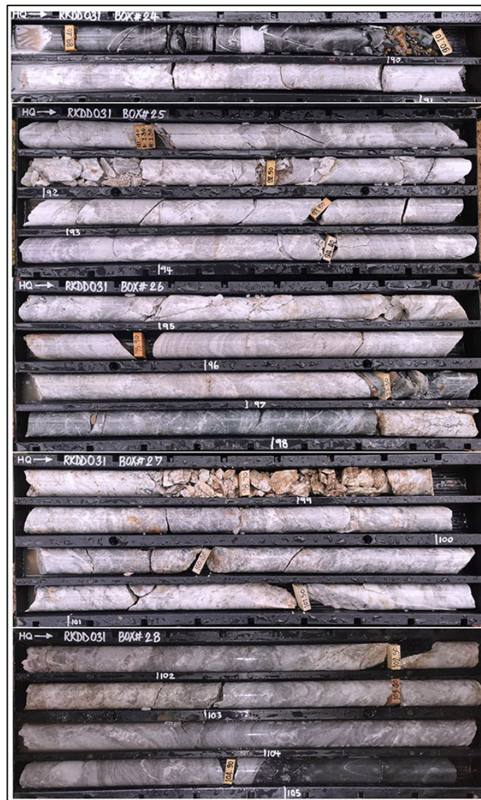
Photo 3. RKDD031 from 90.1 to 104.9m showing pegmatite with lepidolite
