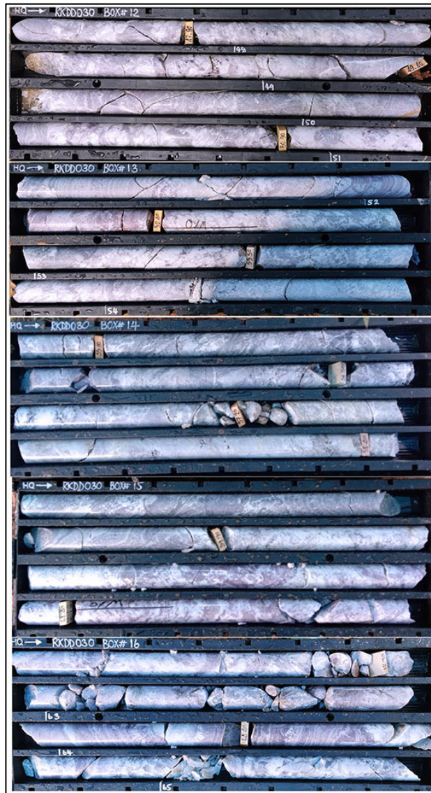
Photo 2. RKDD030 from 47.8m to 65.5m, showing pegmatite with lepidolite
