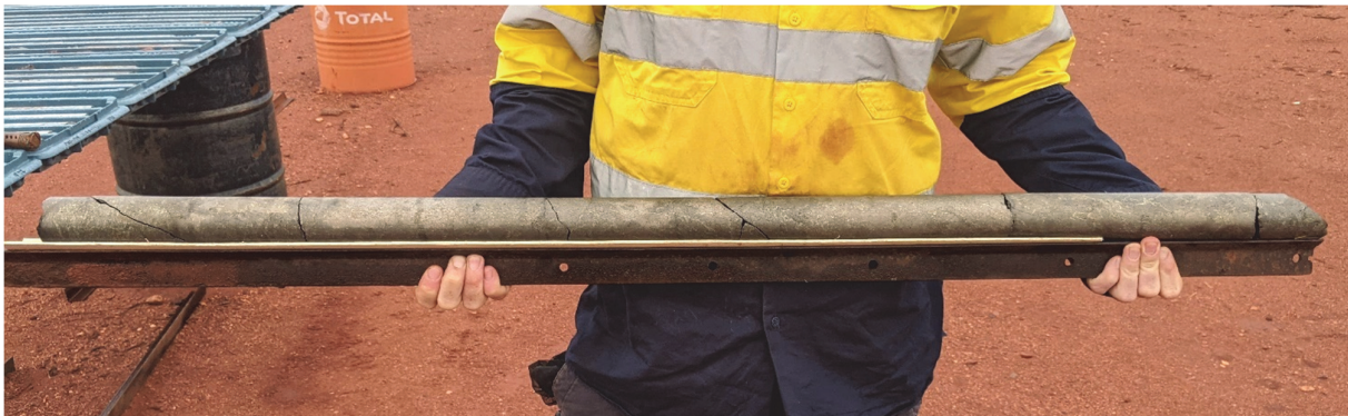
Figure 1 – drill core from the massive sulphide interval of MAD199 between 342.12m to 343.4m downhole.
