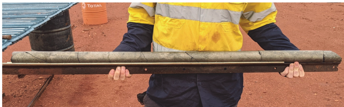
Figure 1 – drill core from the massive sulphide interval of MAD199 between 342.12m to 343.4m downhole.
