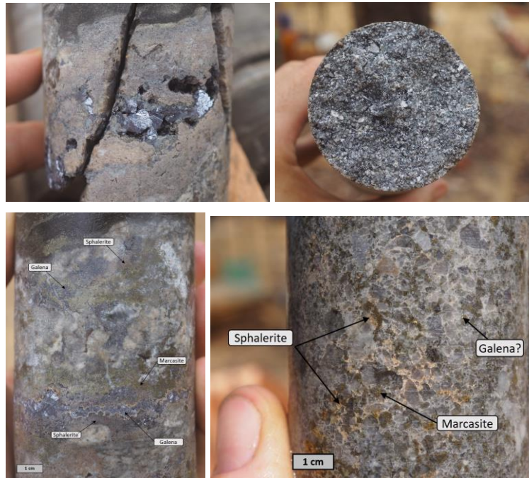
Figure 6: Examples of mineralisation styles being encountered at Niamabimbou
