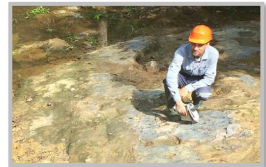
Outcrop of mineralised sandstone at the Dikaki embayment containing approximately 20 – 40 % galena and sphalerite
