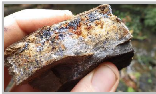
Carbonate hosted mineralisation at Dikaki – showing coarse galena crystals
