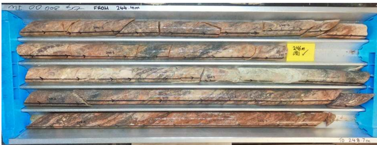
Figure 14: Potassic alteration in drill core from hole MIDD008, 244.4 - 248.7m.
