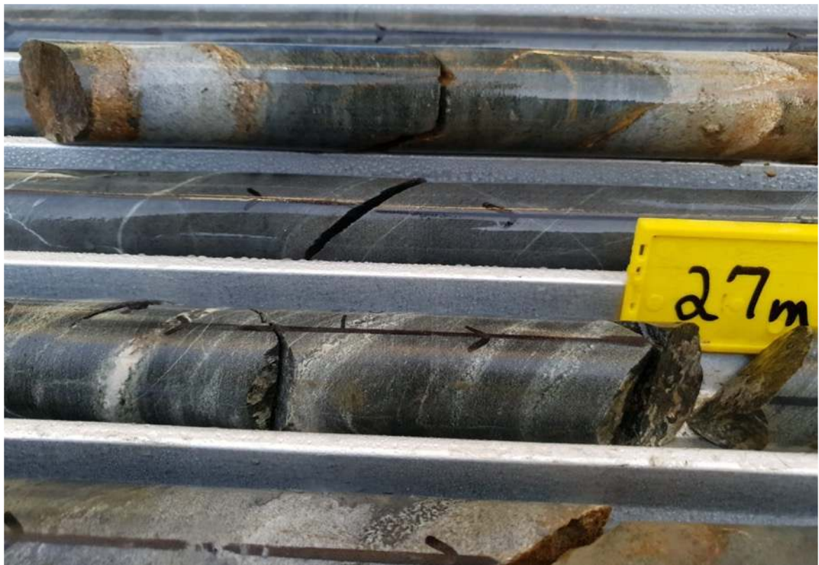
Figure10: Amphibolite with quartz veins/stringers and oxidised sulphides at 27m depth in SODD003.
