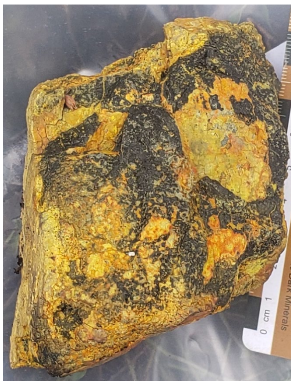
Figure 1: Photo of uraninite float sample found east of the Hook Lake Prospect (Sample # 143826 – 59.2% U 3 O 8 )
