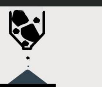
3 **Processing of Kalkaroo sulphide ore** Pyrite concentrate containing 0.3% Co, 2.5 g/t Au, 1% Cu **FLOAT** Roasting of pyrite & leaching of calcine Moly REE Copper Recovery 28%+ 90%+ Gold Copper sulphide concentrate Sulphuric acid Cobalt sulphate product
