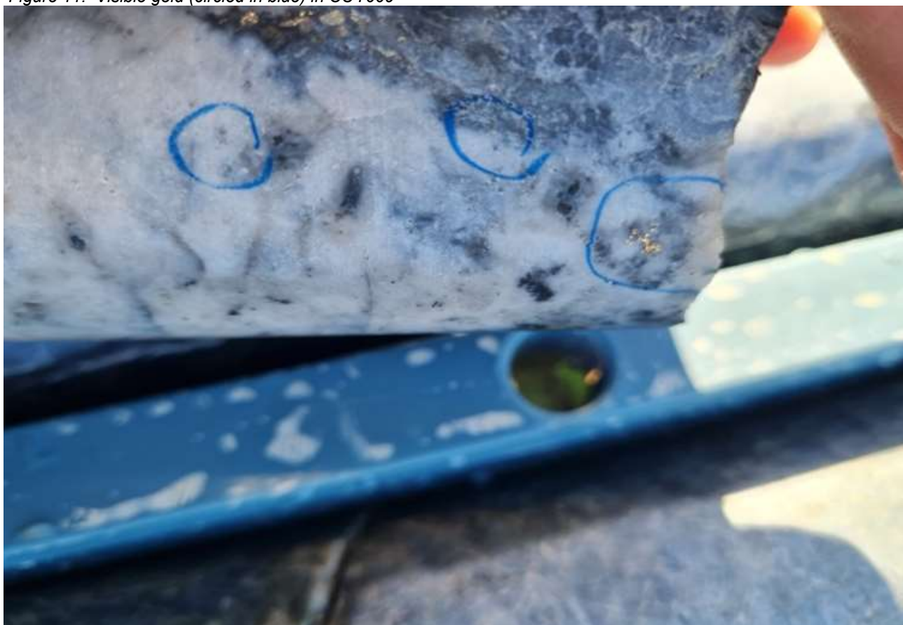
Figure 11. Visible gold (circled in blue) in CUY009
