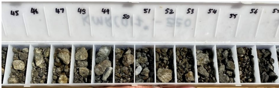
Figure 4: KMRC017 chip tray with semi-massive/massive sulphide (45-57m) assaying 12m @ 1.6% Cu, 31.7 g/t Ag, 0.5 g/t Au from 45m.
