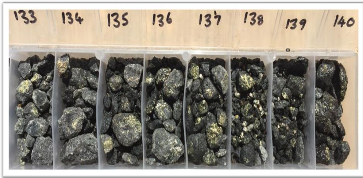
Image 4. RC Drill chips from hole TR17RC07, showing Chalcopyrite with Cobalt mineralisation.
