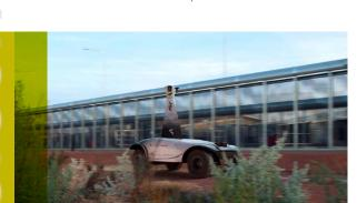
Testing of the perimeter is aided by a robotic actuator that extends out of the vehicle and simulates cutting or climbing of the fence.
