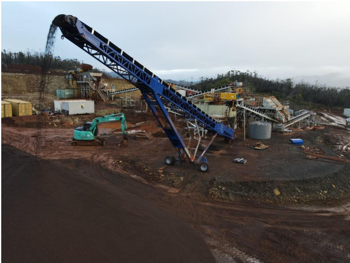
Figure 2 | Radial Stacker delivering Iron Ore product onto stockpile ready for haulage
