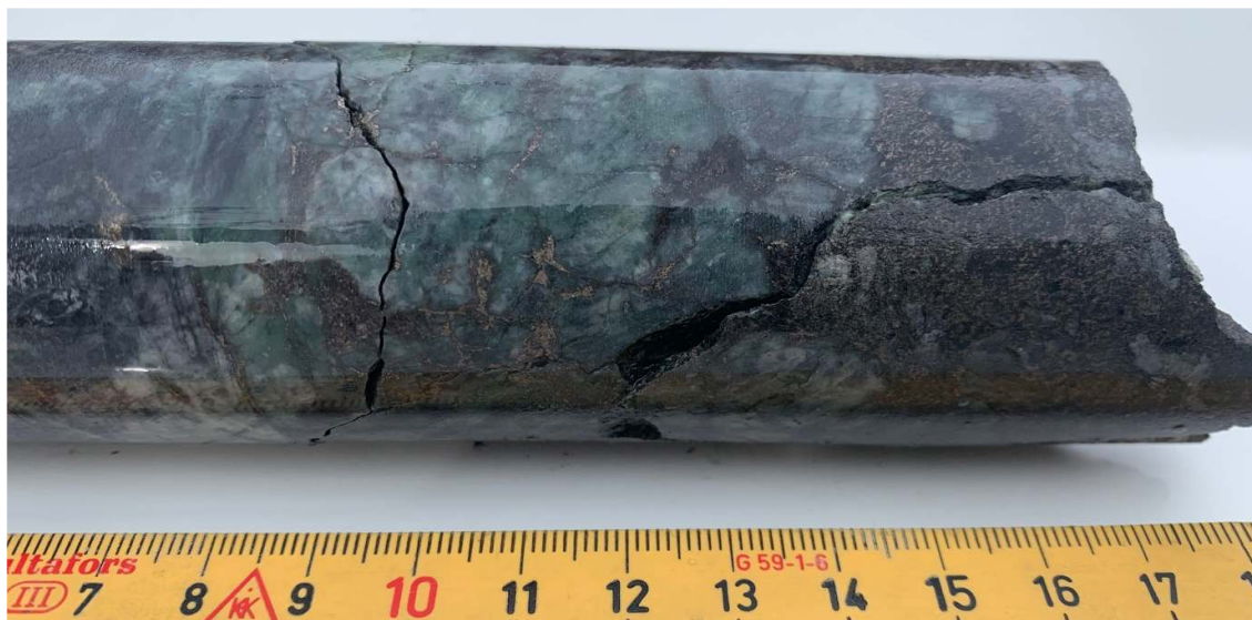
Figure 3 Pyrrhotite mineralisation hosted in metavolcanic within SODD001 from 196.3m downhole.
