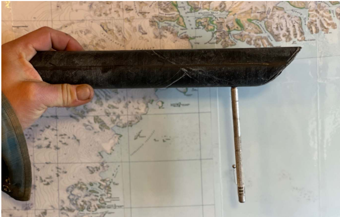
Figure 1 Magnetic pen holding onto magnetite at SODD001 from 196.5m downhole.
