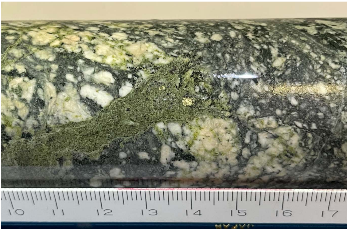
Figure 11 Bleb of chalcopyrite within MIDD007 from 99.8m downhole.
