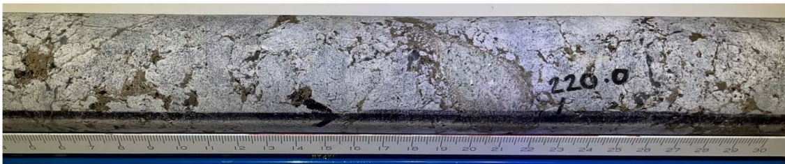
Figure 6 Sulphide and phyllosilicate mineralisation within leached metavolcanic in SODD001 from 219.8m downhole.
