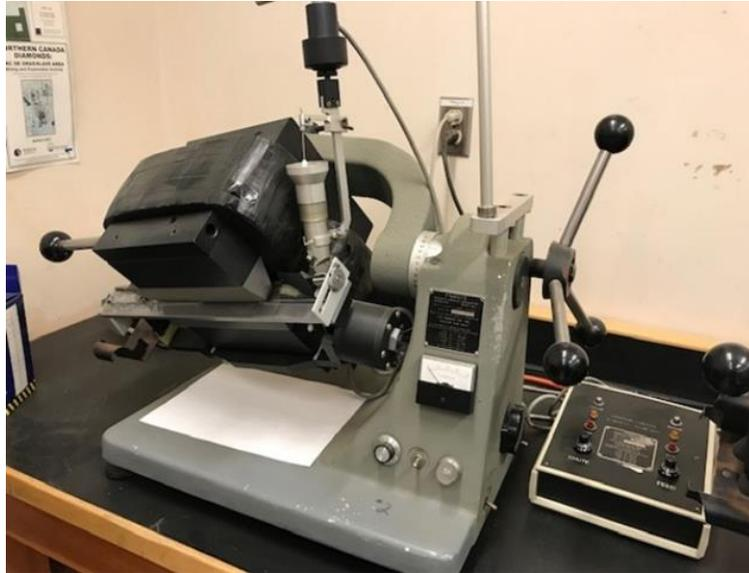
**Figure 2 A Laboratory Magnetic Separator (Frantz)**
