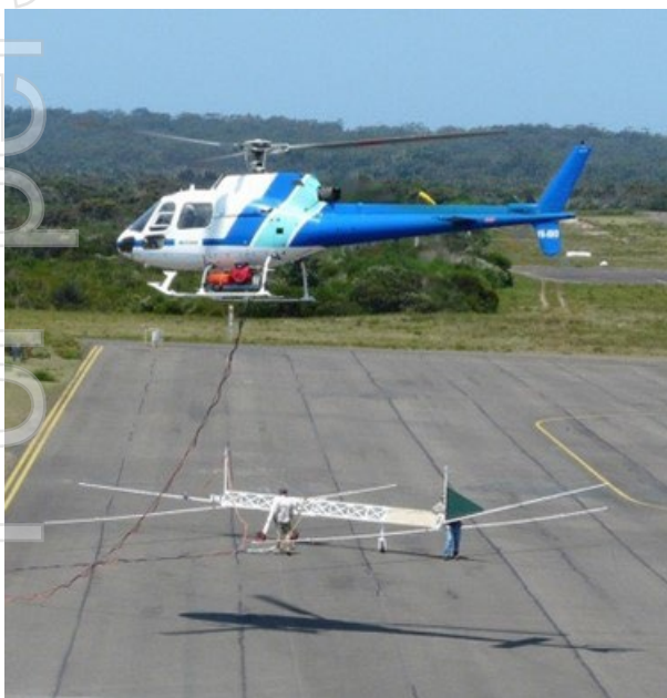
Figure 1: Airborne Geosolutions TDEM REPTM data capture system.
