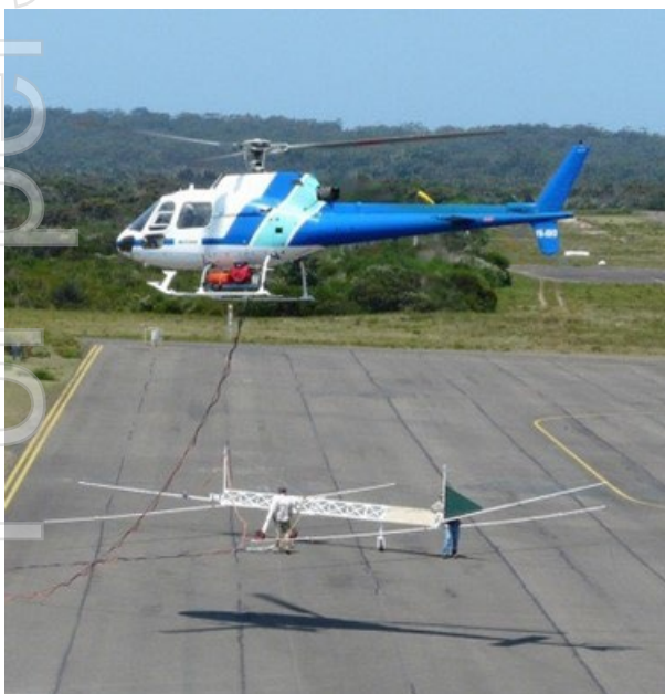
Figure 1: Airborne Geosolutions TDEM REPTM data capture system.
