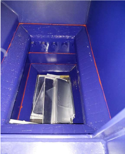
Figure 2 - LIB pouch cells in the feed hopper to the primary shredder
