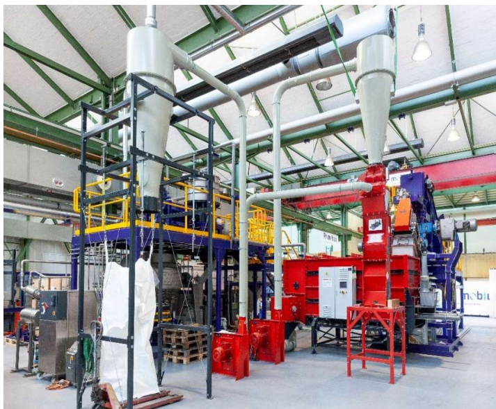
Figure 1 - Profile of the Primobius Shredding and Beneficiation Circuit
