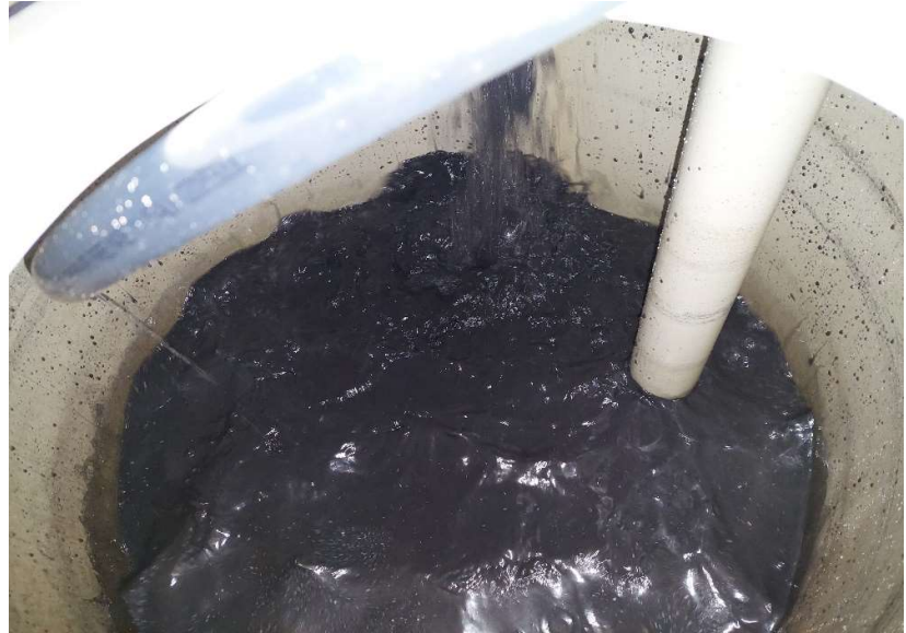
Figure 3 - Shredded material being friction washed to liberate cathode materials from the metal foil electrodes
